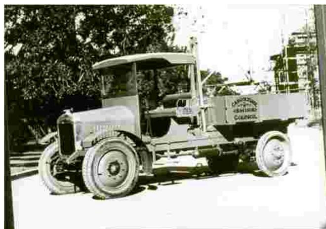
The body of this tip truck was built on a Thornycroft chassis by the firm for the Caboolture Shire Council. It is a heavy duty work horse and needed to be tough. The tray was tipped up by a man turning a crank handle, on the side of the truck, which wound a rope attached to a pulley shown above the back of the cabin.
